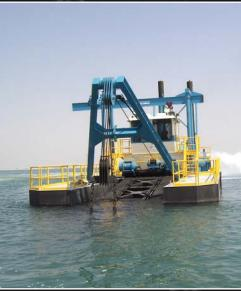
General: all dredges feature a PLC based operating system, electro-proportional hydraulic circuits, hi-capacity service water system, in-line direct marine style transmission for dredge pump reduction, engineered for portability, Caterpillar engines and power up/down spud system. Detailed specifications available upon model determination.
