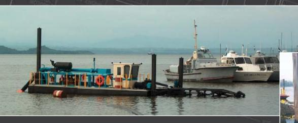
Often called the contractors "dream machine", the Barracuda Class Dredge features a swinging ladder design and is easily transportable. The Barracuda Class dredge is available in both diesel or electric power. Standard Discharge sizes range from 10" (254mm) through 16" (+) (406mm) and the dredge can be customized to your particular needs. The Barracuda dredges have been most commonly used in maintenance and waterway lake revitalization projects.
