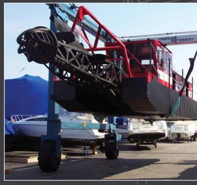
The Badger class dredge is offered in an 8-Inch configuration and features a 250 hp John Deere diesel engine. With a maximum digging depth of 15 feet, this 64' long dredge is ideal for smaller dredging jobs where more compact equipment is required due to work area limitations.
